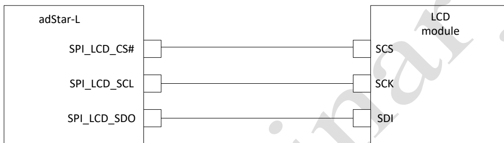
Figure 19-3 9bit mode pin connection
