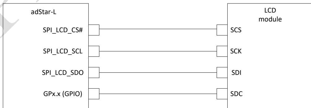
Figure 19-1 8bit mode pin connection
