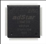
ADChips Corp.'s 32bits Microcontroller, adStar-L has 2KB SRAM for instructions and 1KB SRAM for data. Moreover, LCD Controller is an appropriate General MCU for graphic user interface development.
