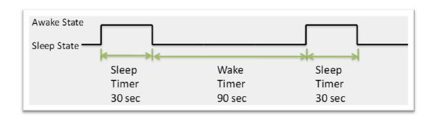
The above diagram shows the transitions between the Sleep state and Awake state based on the sleep and wake timers.
